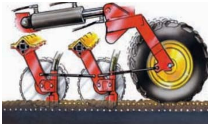
Fig.6 Connecting the furrow forming tools to the rear wheels
