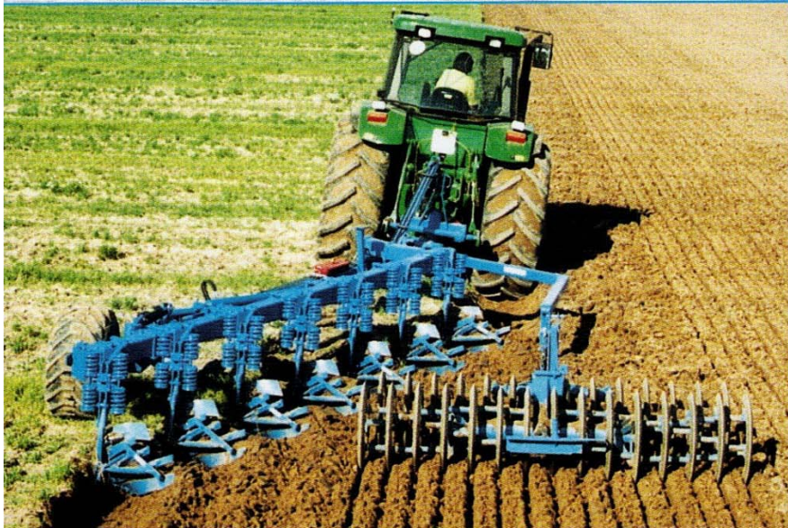
Fig.4 A plough equipped with a clod-breaker
