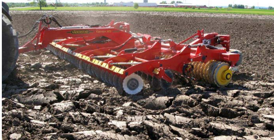
Fig.2 A disc cultivator with a toothed roller
